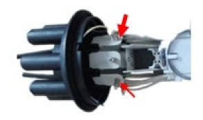
3. Remove the sheath of the cable and clean it.Cut the strengthen member to 5 cm length.Put it through the attach screws and bend it to fix on the screw. Then tighten the screw.
