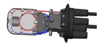
6. Coiling the optic fibers in the splice trays as above picture from the bottom tray to the top one. Fusion the joints and shrink the protective tubes and fix them in the tray. And put on the tray lid.
