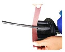
8. Using abrasive strip to rough the surface of the cable sheath and ports slightly.
