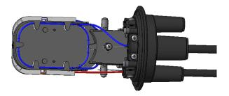
5. Wind the excessive loose buffers in suitable cycles and put in the storage basket.
