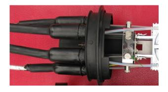
3. Remove the sheath of the cable and clean it. Cut the strengthen member to 5 cm length. Put it through the attach screws and bend it to fix on the screw. Then tighten the screw.
