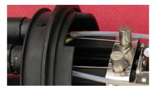
4. Remove the loose tube of the cable and clean the bare fibers. Put them through the transparent PE tube, using PVC tape to wrap the end of the PE tube and cable.
