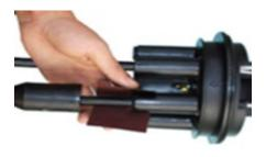
7. Using abrasive strip to rough the surface of the cable sheath and ports slightly.
